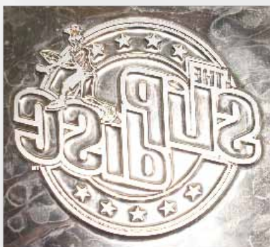
Foil stamping plate for the Slip Disc frisbee (see right) >>
