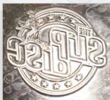
Foil-stamping plate for the Slip Disc (see right)
